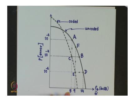
Now the figure out here depicts 2 curves, one curve is for the un-coded system and the other dotted curve is for the coded system. And here we have plotted the probability of error versus signal to noise ratio per bit that is Eb by italic N in dB.
