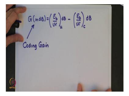
This is equal to SNR per bit required for the un-coded system and difference of this width, the SNR per bit required for the coded system, so this is known as coding gain. So, we get a coding gain of 5 dB for the same error performance, but lower SNR per bit. So, by moving from point D to point E we have lowered the SNR per bit requirement, but again this is done at the cost of bandwidth because, the bandwidth requirement will again be higher assuming real time system.
