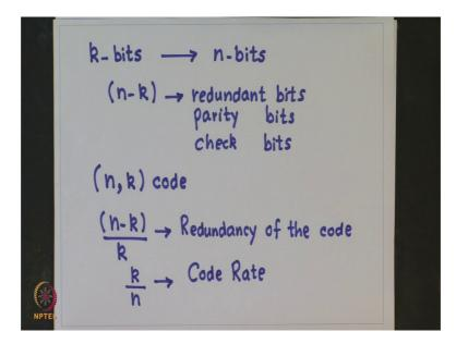
So, we have message sequences of k bits and this gets transformed to n bits sequence, where n is larger than k. Now the n minus k bits which the encoder adds to each data block are called redundant bits are also known as parity bits or check bits and the code is referred to as n comma k code.
