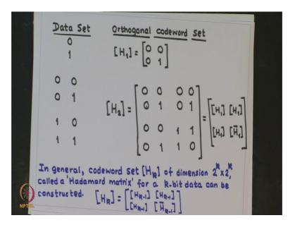
And similarly we can have a 2 bits data set transform using orthogonal code words of 4 digits each described by the rows of matrix H 2. Now H 2 is obtained from the matrix H 1 by this relationship, the bar on H 1 denotes that all the elements in the matrix H 1 are complemented. So, H 1 corresponds to this matrix, so H 1 bar corresponds to this matrix.
