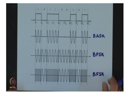
Our binary FSK modulated signal would look something like shown in this figure. So, this is your BASK and this is BPSK which we have studied earlier and this figure out here corresponds to binary frequency shift keying. So, we see that for symbol 1 we have one frequency and for symbol 0, we have another frequency
