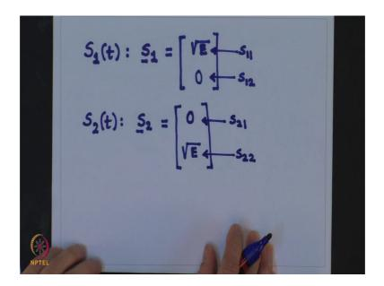
. So, S 1 t would get mapped to S 1 vector and it will have 2 components; the first component in this vector would be root E that is the projection of S 1 t on phi 1 t and the projection of S 1 t on phi 2 t would be equal to 0. So, this is your S 1 1 and this is your S 1 2.
