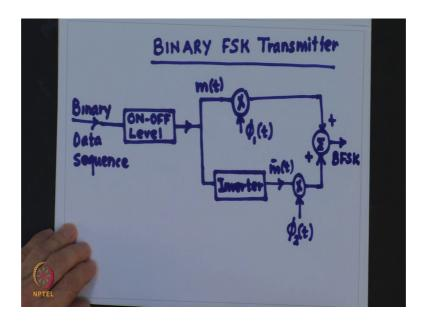
So, binary FSK transmitter would be something as shown in this figure. We have binary data sequence 0s and 1; we pass it through on off level encoder. So, the output of that this becomes my message signal, we multiply this by phi 1 t, we take this pass it through a inverter.
