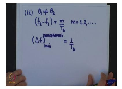
Let us take another case when the 2 phases are different; that means, theta 1 is not equal to theta 2. In that case, again from here it is easy to see that the difference f 2 minus f 1 should be m by T b correct because you will have to take care of this terms, theta 2 is not equal to theta 1. So, this sin terms have to get cancelled and that is why we get that relationship is simple to see that m is equal to 1 2 and so, on.
