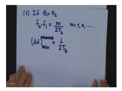
. So, first is if theta 1 is equal to theta 2, we get the condition that f 2 minus f 1 should be equal to m by 2 T b where m is equal to 1, 2 and so on. So, the minimum frequency separation f 2 minus f 1 for orthogonality will occur when m is equal to 1 and then in that case this separation is indicated as follows minimum is equal to 1 by 2 b.
