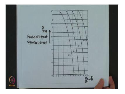
So, this curve clearly shows that an M keeps on increasing correct for a particular value of symbol error, the E b by italic n ratio also keeps on increasing, or for the same value
