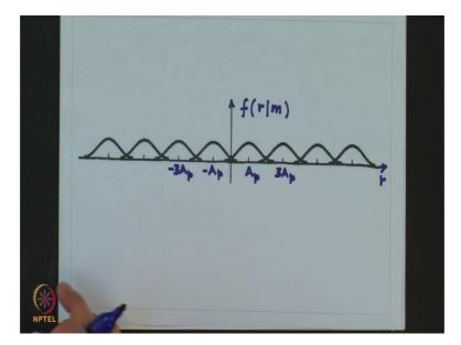
And the signal consolation for this will have is of the form. This corresponds to plus p t, this corresponds to minus p t, this corresponds to the 3 p t, and this corresponds to minus 3 p t. So, signal constellation which is nothing, but the representation of the message signal in the orthonormal basis signal, which in this case is nothing, but the pulse itself p t divided by the root of it is energy ok.
