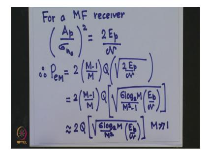
Now, let us calculate this quantity we know for a match filter receiver. This ratio squared is equal to twice into the energy of the pulse italic N italic N by 2 denotes the power spectral density of the white noise. Using this relationship, we get the probability of symbol error to be, using this relationship for the average energy and the energy of the pulse, we can rewrite this as.
