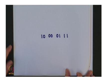
I have 0 0 this could be 0 1 this is 1 0 correct and the next 1 is a 1 1. So, difference if you take the adjacent difference, there is a difference of only 1 bit. So, that happens basically if you assume, then in this case the probability of bit error would be equal to symbol error divided by log of M to the base 2 fine. And if you do this and, if you plot this is the kind of curve which we get.
