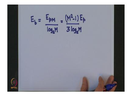
So, from this we can calculate the average bit energy which is equal to the average, energy in the pulse the number of bits which each pulse carry the information is log to the base 2 M all are of equiprobable. So, this is equal to M squared minus 1. Now, it is important to note that for a given information rate M-ary PCM bandwidth is less than that of the binary PCM by a factor of log of M to the base 2. Now, let us try to calculate error probability for this M-ary PCM.
