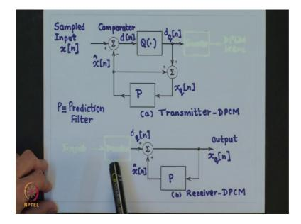
So, let me just show you this right which we had studied last time also. So, this is a transmitter end of the DPCM and this is the receiver end of the DPCM and we have this block which we call it as a prediction filter block, which is there both of the transmitter end and at the receiver end. And what we are interested is basically to get a good predictor so, this variance of this difference sequence can be substantially reduced.
