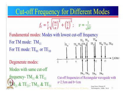
Now, let us see the graph of cutoff frequencies this plot represents the cutoff frequency of a rectangular waveguide with a is equal to 2.5 centimeter and b is equal to 1 centimeter. So, for TE 1 0 mode, the cutoff frequency for this waveguide comes out to be 3 gigahertz; for TE 2 0 mode, it is 6 gigahertz. Similarly, for other mode, we can calculate in this the lowest cutoff frequency is of TE 1 0 mode.
