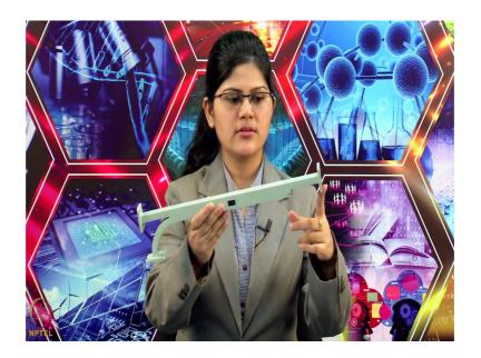
So, in this is the input port, this is the through port this is the coupled port and this is the isolated port, this isolated port in this coupler is terminated with a mesh load this coupler is a 10 dB coupler. So, if we give input 0 dB here, then we will get minus 10 dB here at the coupled port.
