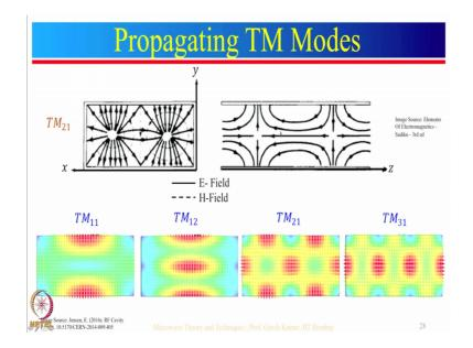
This is the example for TM 2 1 mode, this graph is for xy plane, this is the variation of fields in y z plane. So, as you can see from this, there is A 2 half sinusoidal variation of the fields in x direction and there is only one half sinusoidal variation of the fields in y direction. In general, an TM mn mode there is m half sinusoidal variation of fields along x direction and there are n half sinusoidal variations of the fields in y direction.
