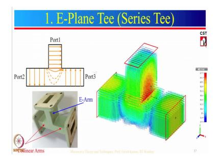
So, first we will have E-plane Tee and E-plane Tee. This is the port one which is called as E-arm this is port 2 and this is port 3. These 2 are called as collinear arms, if input is given to port number 1, then the power will be divided in these 2 ports, but the outputs at these ports will be 180 degree out of phase as you can see from this figure if the direction
