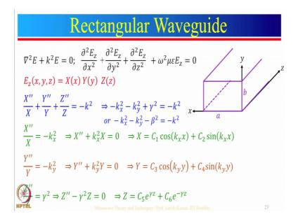
In rectangular waveguides, there are 4 finite metallic plates of which 2 metallic plates are in yz plane and those plates are separated by a distance a in x direction and the 2 metallic plates are in xz plane which are separated by a distance b in y direction.
