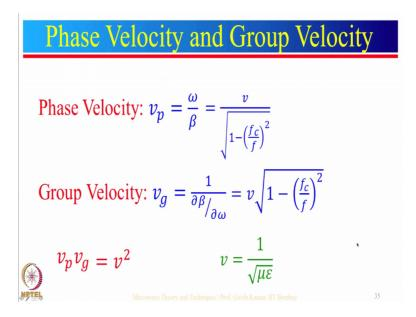
Now, let us see the phase velocity and group velocity the phase velocity as we have discussed earlier that it is given by omega by beta. So, if we put the value of beta here, then we will get the phase velocity vp is equal to v divided by under root 1 minus fc by f whole square similarly we can calculate the group velocity which is equal to 1 upon dou beta by dou omega by solving this, we will get v into under root 1 minus fc by f whole square.
