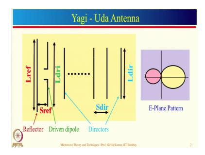
So, Yagi-Uda antenna consists of one driven dipole, which you can see over here. And then, we have a one reflector behind the dipole, and then after that we have multiple directors on the other side. So, what is the purpose of all of these thing. Now, we have covered that a dipole antenna has a radiation pattern which is omnidirectional radiation pattern. So, it will radiate equally in all the direction.
