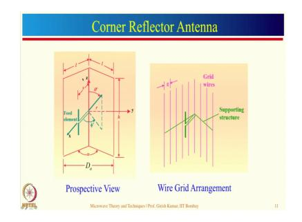
Now, let us go to the next configuration. So, we will start with corner reflector antenna. So, corner reflector antenna is defined by its angle alpha between the two metallic plates over here. Now, generally speaking these metallic plates are defined by the height and the length of each section. So, most of the derivations in the book, assume h to be infinity and l to be infinity. However practically that will never be the case. So, let me give you some practical tips over here.
