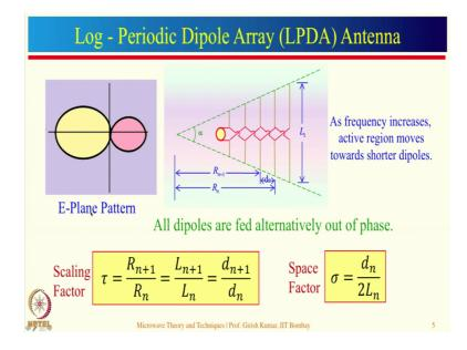
Now, let us talk about log-periodic dipole array antenna. Here, purpose is different than the Yagi-Uda antenna. In case of Yagi-Uda antenna, we try to increase the directivity of the antenna, whereas bandwidth is relatively limited. However, in case of log-periodic, more emphasis is given on the bandwidth. So, here all the dimensions of the dipole antenna vary logarithmically. So, let us see what the configuration is. So, here we have a one dipole, another dipole, another dipole and so on.
