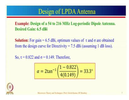
So, we are taking a design example of a log-periodic dipole antenna array from 54 megahertz to 216 megahertz. Let us say the desired gain is equal to 6.5 dBi. Now, as I mentioned for gain equal to 6.5 dBi, choose the optimum values of tau and sigma for directivity equal to 7.5 dBi, assuming 1 dB loss. So, we can read these values of tau and sigma from the previous curves, so tau is about 0.822, and sigma is 0.149. So, from here, we can also calculate the angle of the dipole antenna array.
