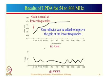
So, let us see the result of this particular design. So, you can see that this is gain versus frequency, this is VSWR versus frequency. So, one can see that VSWR is less than 2 over this entire band. Now, let us see gain. Gain as you can see here, gain is relatively small at the lower frequency, whereas gain is (Refer Time: 15:41) at the higher frequency. The reason for that is behind the longest dipole element, there is a nothing which is reflecting back.
