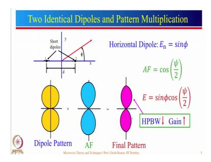
So, now, instead of taking isotropic elements, let us take horizontal dipole over here and horizontal dipole over here. So, 4 horizontal dipole, we know that maximum field will be in this particular direction just recall I have mentioned to you, that you can think about a dipole as a pen.
