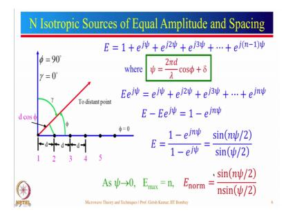
So, now instead of using 2 elements, if we use N elements so, here are N elements. So, you can start from 1 2 3 and so on. Here, we have taken the first element at origin and then other elements are at equal distance which is equal to d. So, now, we can find out the E, which is far field pattern, because of all these elements we can find the total field at a faraway distance.
