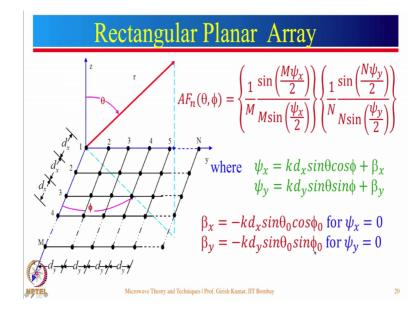
Now, we will shift to the next configuration, which is rectangular planar array. So, here we have n elements along this particular axis. And, there are m elements along x axis. So, distance between the elements along the x axis denoted by d x d x and d x. And, along this particular direction distance between the elements is dy dy all these elements have equal distance. So, now, let us see how we can find out the overall radiation pattern for this rectangular planar array?
