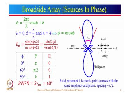
So, this is a broadside array in which all the sources are fed in the same phase. So, 4 example here, we have 4 elements distance between all the elements is equal to d. So, we know that psi is given by this expression, but since they are in same phase delta will be equal to 0.
