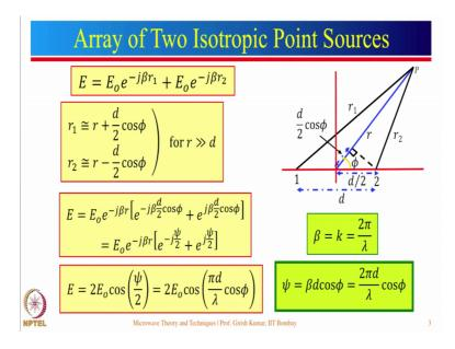
So, let us start with array of 2 isotropic point sources. So, we have a source 1 over here and there is a source 2 distance between the 2 elements is d. And these 2 elements are centered around the origin so, this distance is d by 2 this is also d by 2. Now, we want to find out the field at a point P, which is at a distance of r from the origin. And, distance from the 2 elements is r 1 and r 2.
