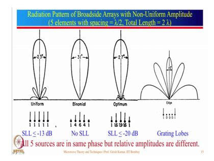
For this particular case the problem is that side lobe levels are less than minus 13 dB or so in fact, in fact even for a very large uniform array side lobe level can be at best 13.5 dB. There are many applications where we would like side lobe level to be less than 20 dB or less than 30 dB. So, you can see that for 5 elements fed with equal amplitude and equal phase half power beamwidth is of the order of 23 degree, but side lobe levels are of the order of 13 dB.
