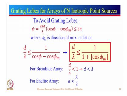
Now, I am going to talk about what is grating lobe and how we can avoid these grating lobes? Ok. So, to avoid grating lobes, we have to put the condition that psi should be always less than or equal to 2 pi. We had seen that beam maxima comes for psi equal to 0, but again beam maxima comes when psi becomes equal to 2 pi. So, if we maintain this condition that psi should be always less than 2 pi, then we can avoid grating lobe.
