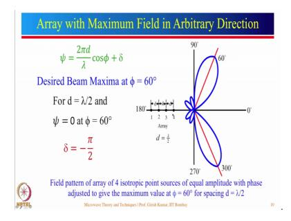
Now, let us see array with maximum field in arbitrary direction. So, let us say we want desired beam to be along phi equal to 60 degree. So, how do we find the value of delta well? Let us say for d equal to lambda by 2 what we need to do we put the condition psi equal to 0 at phi equal to 60 degree.
