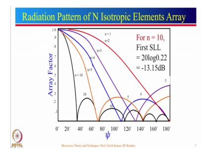
So, here is a radiation pattern of n isotropic elements array so, for n equal to 1 will have simply this kind of a pattern for psi varying from 0 to 180 degree. So, when n is equal to 2 it varies from 1 to 0. So, for n equal to 3 you can see there is a null over here, at this particular thing is known as side lobe level. As, n increases you can see that half power beamwidth is decreasing, half power beamwidth will correspond to which point. So, this
