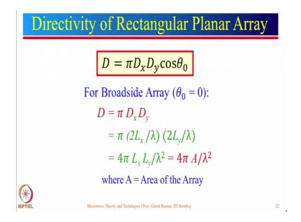
So, now let us see how to find the directivity of the rectangular planar array? So, to find the directivity of the planar array all you need to do it is use this particular expression, where D x is the directivity along the x axis for the linear array D y is the directivity of the elements along the y array.
