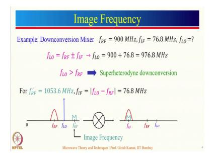
Now, let us take an example of a downconversion mixer. Let us say that, we have an incoming frequency at the RF band, which is equal to 900 megahertz. And the IF desired is 76.8 megahertz. And the question is the LO frequency that is required to produce this conversion. Simple, we have a formula f LO is equal to f RF plus or minus f IF using the basic mixer operation. Now, if I choose the plus sign here, I get the local oscillator frequency to be 900 plus 76.8, which is equal to 976.8 megahertz.
