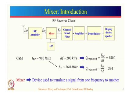
Let us take an example of an RF receiver chain, where we have an antenna, which receives the signal. And we have an RF amplifier, which amplifies the signal, then we have a channel select filter, and the signal is further processed using amplifier, demodulator, and then finally given to a display or a speaker. Now, let us take a case of a GSM mobile system, where the incoming signal is at a frequency of 900 megahertz. And the channel select filter requires a bandwidth of 200 kilohertz.
