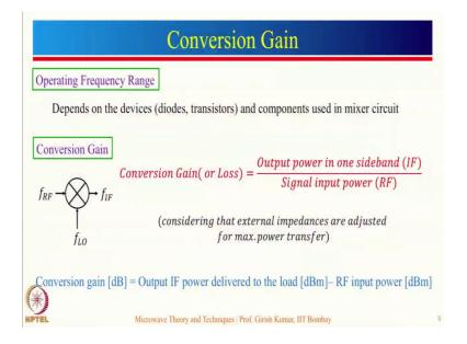
So, before going to the conversion gain, let us first discuss about the operating frequency range of a mixer. And it depends on the devices, which are nothing but diodes and transistors that are used while building the mixer, and also depends on other components that have been used to build the mixer circuit. Conversion gain very simple, it is defined as the output power in one of the sidebands, which is the IF output power divided by the RF input power.
