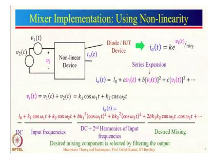
So, let us take the case of mixer implementation using non-linearity. So, here you can see, we have a non-linear device. And we know that, it can be a diode or BJT, at the input we have a signal v i and the output we have a current, which is i o. Now, we know that the diode current and voltage relation. So, the output current varies exponentially with the input voltage. And if I expand this particular expression using a Taylor series, what I get is this expression.
