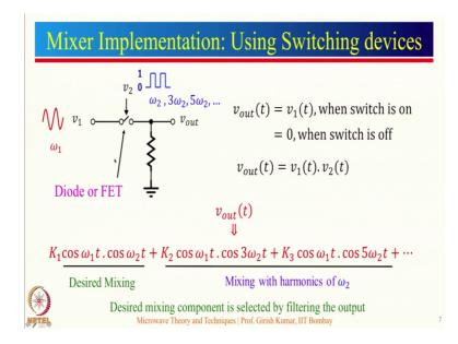
Let us take the 2nd case, where we have mixer implementation using a switching device. So, in this case, you have a input sinusoidal signal v 1, which is given to the output through a switch, which is controlled by the second signal v 2, which is typically a square wave ranging from 0 to 1. So, the input is switched to the output using a control signal v 2. So, simply v out is nothing but v 1, when the switch is on. And it is equal to 0, when the switch is off.
