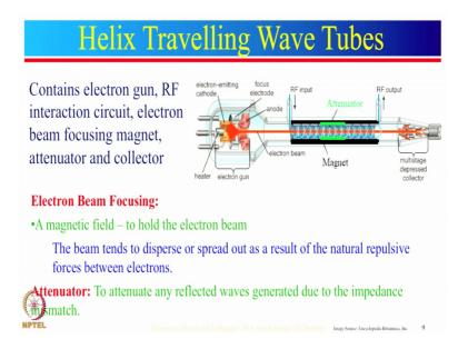
In general helix travelling wave tubes contains a electron gun and RF interaction circuit and electron beam focusing magnet and attenuator and a collector. Let us see these things one by one.
