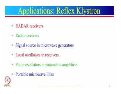
Now, let us look into the applications of the reflex klystron. There are many applications of reflex klystron such as they can be used in radar receiver. They can be used in radio receivers or in signal sources in microwave generators. They are also used in local oscillators and receivers, or in pump oscillators and in parametric amplifiers. And these are also used in portable microwave links. So, these are all applications of reflex klystron.
