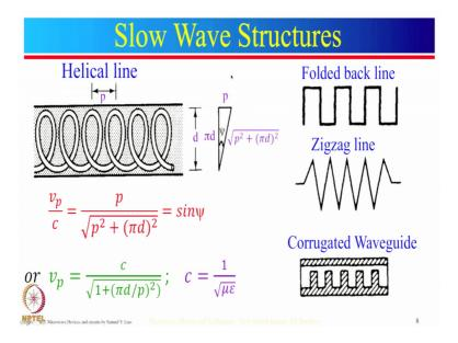
This job is done by slow wave structures. There are many slow wave structures such as helical line, folded back line, zigzag line, corrugated waveguide and so on. And what happens in these slow wave structures is that we provide a larger path length for a electromagnetic wave to travel from one point to another as compared to the electron beam path that is the shortest path.
