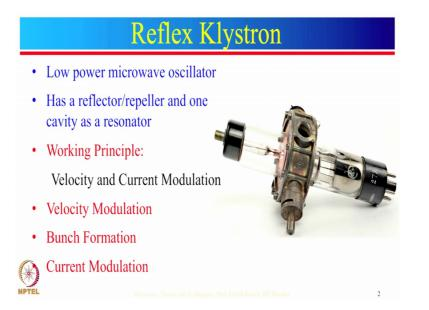
It is a low power microwave oscillator. And to design a oscillator, the first thing which we need to know is how oscillations are generated. The answer to this question is that we need to give positive feedback from output to input such that the loop gain is unity or we can say for a klystron if a fraction of output power is feedback to the input cavity such that the loop gain magnitude is 1 and the feedback path phase shift is 2 pi or multiple of 2 pi, then the klystron will oscillate.
