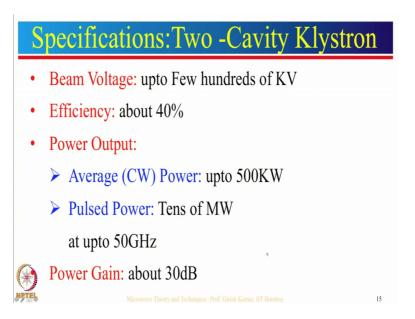
Now, let us see the specifications of practically available two-cavity klystrons beam voltages up to few hundreds of kilovolts can be given. The efficiency of practically
