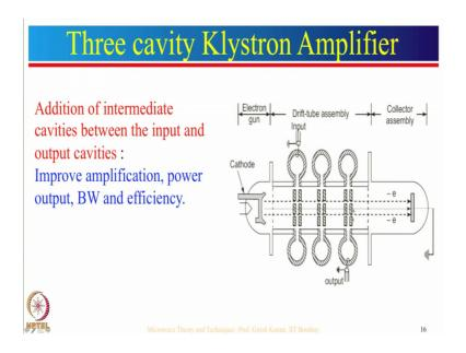
For example, in three cavity klystron, there are three cavities. One is input cavity, another one is output cavity and between these two there is a reentrant cavity. This reentrant cavity increases the output power bandwidth and efficiency of this three cavity klystron amplifier.
