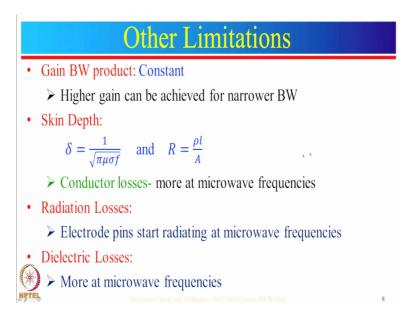
Now, let us move onto the next limitation which is gain bandwidth product limitation. At microwave frequencies the conventional tubes start resonating; and for a resonant circuit
