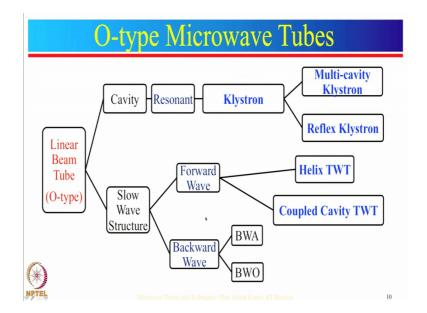
Now, I will discuss classification of linear beam tubes. Linear beam tubes are of two types, cavity type and slow wave structure type. Cavity type structures are the resonant structures; and slow wave structures are the non resonant structures. Each one of these structures have some advantages and some disadvantages which I will discuss after covering these two structures.
