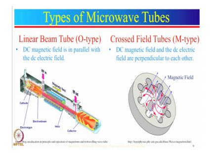
Now, I will start microwave tubes. Microwave tubes are of two types. One is linear beam tube or O-type tube and the second one is crossed field tubes or M-type tubes. In M-type tubes DC magnetic field and the DC electric fields are perpendicular to each other as shown by this figure.
