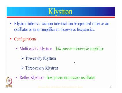
So, let us start with klystron. So, klystron tube is a vacuum tube that can be operated either as an oscillator or as an amplifier at microwave frequencies. In klystron, there are two configurations one is low power microwave amplifier which is multi-cavity klystron; and another one is low power microwave oscillator which is reflex klystron.
