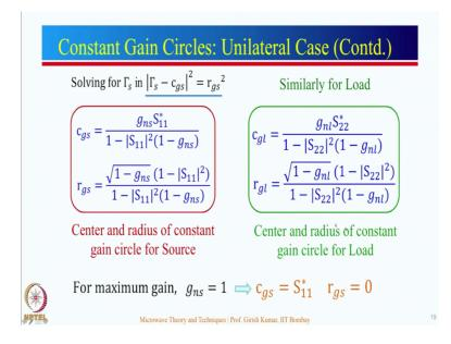
Then, we found out equation of a circle for both source and load.
