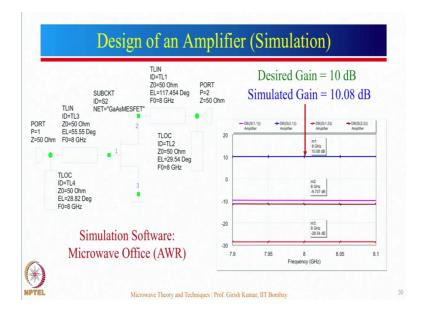
So, we have used microwave office software and we have done the simulation of this particular amplifier. You can see that these are the various simulated parameters. So, this is the device over here, this is that transmission line, this is that stub over here, then the transmission line stub, ok.
