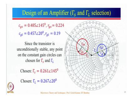
So, now we have to plot the constant gain circle. So, let us see for the source site c gs is 0.485 angle 145 degree. So, you draw a line like this which is at an angle of 145 degree and then, choose 0.485. As I mentioned if you assume this distance is approximately 10 centimeter which corresponds to 1, then 0.485 will be equal to 4.85 centimeter. So, you look at this particular point which will be c gs, then 0.224 is the radius. So, you draw a
