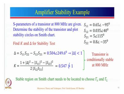
After that we started with an example. For that example S-parameters were given at 800 mega hertz and we found out that this particular transistor is unstable or we call it conditionally stable at 800 mega hertz. The reason for that is delta is less than 1, but K is not greater than 1. In this case, K was less than 1.
