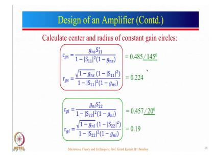
Now, we calculate centre and radius of constant gain circle. So, the expressions are given over here. So, substitute various values for g ns, S 11 we can find out the value of c gs to be equal to this r gs is given by this value. Similarly we find out the values of c gl and r gl. Next stub would be to plot these things on the Smith chart.
