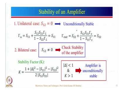
Now, amplifier has to be stable. If amplifier is not stable, then in that case it can become an oscillator. When we talk about oscillator, then we will talk about unstable amplifier, but here we talked about unilateral case in that case S 12 is equal to 0 that would be unconditionally stable. Second cases bilateral case where S 12 is not equal to 0, then we have to check stability of the amplifier and had told you this expression for K. Today I will tell you how this expression of K is derived.
