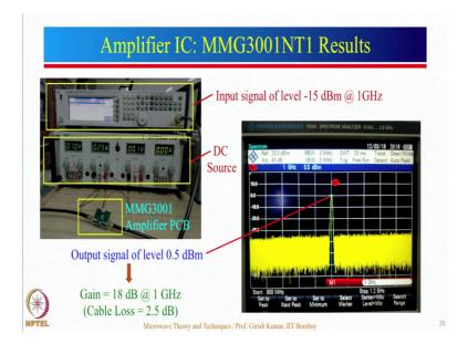
So, here is that amplifier. You can see how small it is and this amplifier input is given from a microwave generator input signal level of minus 15 dBm is given at 1 giga hertz. This is the DC source which gives voltage and current of course and the output of this generator is given as input to the amplifier and output of the amplifier goes to the spectrum analyzer which is not shown in this particular picture.
