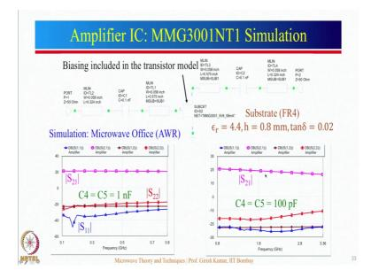
We have simulated this particular circuit using microwave office. So, this is the simulated circuit. So, this particular circuit has been simulated for two different sets of frequency. This is from 0.1 to 0.8 gigahertz and this is from 0.8 gigahertz to more than 3 gigahertz. I just want to mention here the coupling capacitors are taken different in these two cases.
