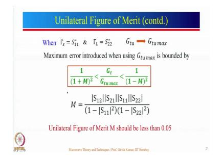
Then, we get this particular range for G t divided by G tu max and when we obtain this, when we substitute gamma S is equal to S 11 conjugate and gamma l is equal to S 22 conjugate where the expression for M is given by this particular terms over here, what you can see over here all these things are magnitude now and also these are only S parameter. So, there is no gamma S or gamma L coming into picture. Why? It is because we have assumed this particular condition.
