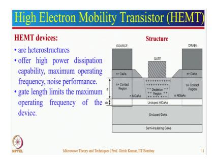
So, there is a improvement on transistor by making the changes in the channel. So, they are known as high electron mobility transistors they are made of heterostructures. In
