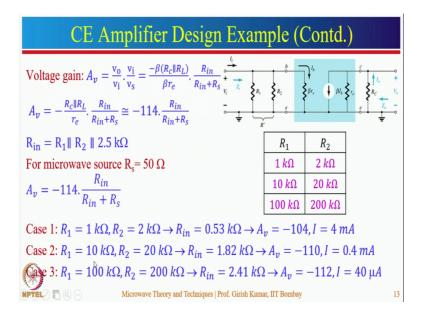
So, here I have drawn the R E model of this transistor. So, the input impedance will be the parallel combination of R 1 R 2 and beta R E. So, beta R E is because of the transistor. So, if you see here and put the value of beta and R E, you will get this particular expression.
