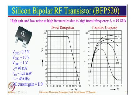
Till now, we just discussed about the operation of the bipolar transistor. So, here is the example of the practically available RF transistor; its name is BFP520. It provides higher gain and low noise and it the transition frequency of this transistor is 45 gigahertz. So, it is fairly good. Now, as I mentioned that the performance of this transistors degrade with temperature; so, here I have shown the variation of the power with respect to temperature.
