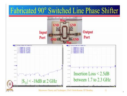
So, letus see the measured results. So we have fabricated a 90 degree switched line phase shifter. So, one can actually see here this is input, that is the output over here, you can see that this is line length 1 1, this is the line length 1 2 and this is the biasing circuit given to this particular circuit.
