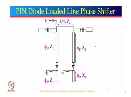
So, this is the circuit realization of a loaded line phase shifter, it also shows the biasing circuits. So we have here input, output and you can see here this voltage is connected through the resistor; which limits the current flowing through these pin diodes. There is a large inductor over here, which acts as a short circuit at dc frequency, but acts as an open circuit at AC frequency.
