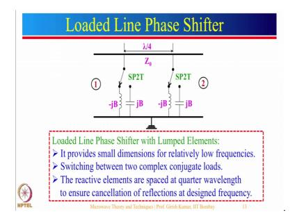
Now, let us look at another type of a phase shifter, this is known as loaded line phase shifter. So, what we have over here? So this is the input port that is the output port. Here we have a 1 S P 2 T switch, another S P 2 T switch and in between we have a line length of lambda by 4. So, let me explain; what is the purpose of this line length over here?
