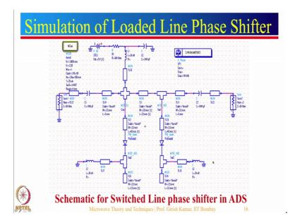
So, let us see the result of this particular configuration. Again it shows the complete biasing circuit over here, one can see that there is a source here, resistor inductor and then there is a diode here the path to the ground is provided through the inductor here, you can see here there is a this additional line length is provided.
