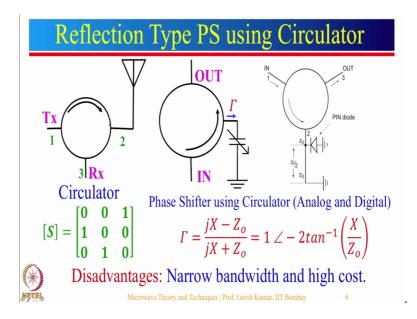
Here reflection type phase shifter is realized using circulator, let us quickly look at what is a circulator? So, circulator is a 3 port device. This arrow direction is very very important. So, this is one of the application not related directly to the phase shifter, but circulators are used for this particular application very commonly.
