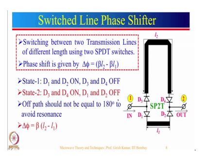
So, let us just take an example of a switched line phase shifter. So, here we have an input at this particular point. This is the output it uses 2 S P 2 T switches. So, this is the 1 S P 2 T switch, this is another S P 2 T switch.
