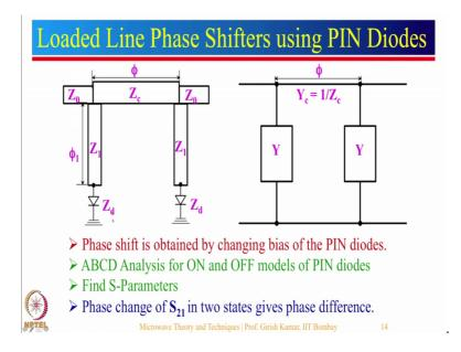
Let us see now, how we can realize lumped elements using a transmission line and pin diode. So, this is just the representation not the actual circuit. So what we have here? This length here will be approximately equal to lambda by 4 after desire frequency, here is a 1 transmission line another transmission line here, which is connected with a pin diode over here.
