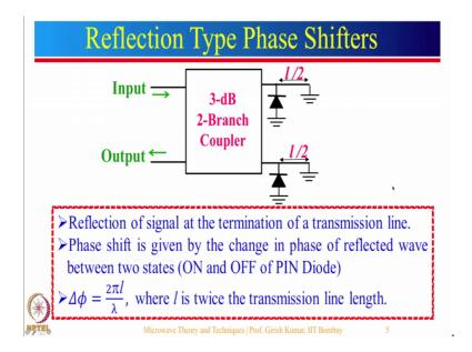
So, now let see, how we can realize these phase shifters. So, let first look at reflection type phase shifter and here we have input coming to one of the port of 3-dB 2-branch coupler, this is the output, the other 2 ports you can see over here that pin diodes are connected over here with the line length 1 by 2. So, let just look at the concept point of view what really happens here.
