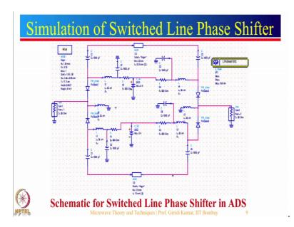
So, we have done the simulation of this particular configuration using ADS software. So, it actually shows a complete biasing circuit also. So, one can see here this is the D C
