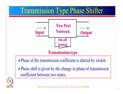
Now, let us talk about transmission type phase shifter. So basically, transmission type phase shifter you can see here there is a 2 port network, we have an input on one side, output on the other side and by controlling the switch position we can change the phase between; the 2 states. So, the phase difference will be realized; when the switch position changes from on to off or off to on.
