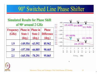
So, let see what is the result of this particular simulation. So, here I have shown you the simulated results for phase shift, we had designed this phase shifter at around 2 gigahertz frequency for 90 degree phase shift. So, in the 2 states this is the S 2 1 phase response plot, here are the values. So at 1.9 to 2.1, we have obtained differential phase shift as 85 90 and 95d egree.
