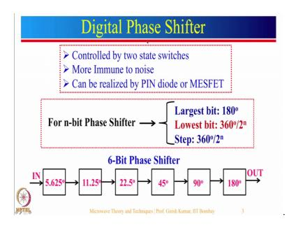
Then we briefly looked at digital phase shifter and for n bit phase shifter largest bit is 180 degree lowest bit is 360 degree divided by 2 to the power n and each step is given by 360 degree divided by 2 to the power n. Then we took an example of 6 bit phase shifter.
