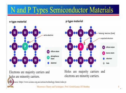
If, we add the impurity of phosphorus in silicon lattice, now we know in case of phosphorus, it contains the 5 electrons in it is outermost shell. So, these electrons form the covalent bond with the silicon lattice that can be seen from this particular figure. And, the 5th is loosely coupled to this lattice.
