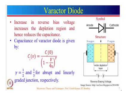
The next diode that we will talk about is the varactor diode. Now, if we see the PN Junction diode and if we try to see the reverse bias behavior of this diode, it shows a very interesting property just to explore that particular behavior just connect the PN junction diode in a reverse polarity. So, that the positive terminal is connected to the N-region and the negative terminal should be connected to the P-region.
