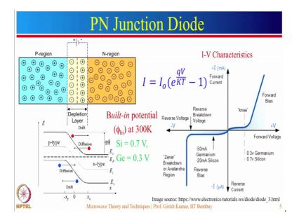
Here you can see that in case of P-region the Fermi energy level is near the valence band, in case of n region the Fermi energy level is near the conduction band.
