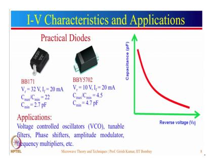
Next, I will talk about the IV characteristics of this diode as I mentioned earlier capacitance decreases with increase in reverse bias voltage. So, this shows the characteristics of the varactor diodes.
