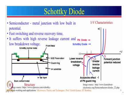
But in this case the junction should be made using the n type of material and the metal. So, in this case the n type of epitaxial layer is deposited on the highly doped n type of substrate and then metal is deposited on the n type of epitaxial layer.
