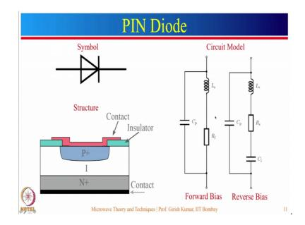
So, the high layer is deposited only on highly doped substrate. And then highly doped P type of subs layer is deposited on the intrinsic region. So, this is how the geometry of this structure is made? Then again the contacts are made to make the connection with the electrical circuit.
