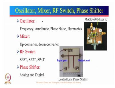
Then we will talk about the various other things which are integral part of any RS system. So, oscillator you can thing oscillator as nothing, but also a microwave generator and we are talking about a microwave generator, there are different things which are important what is the frequency at which it is oscillating of course, there are other things are there which are known as VCO voltage controlled oscillator.
