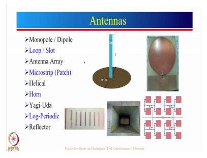
Then we will talk about several antennas in this particular course, we will talk about monopole antennas dipole antennas loop slot antenna; antenna array, micro strip; patch antenna, helical, horn, Yagi-Uda, Log-periodic and reflector antenna. So, just to show you, this is a monopole antenna which is generally considered as a lambda by 4 length over infinite ground plane, but majority of the time the size of the ground plane will be small.
