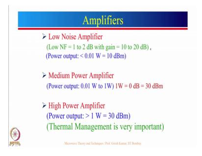
We will talk about several different types of RF amplifiers. So, here we have a loan wise amplifier most of the time these low noise amplifiers will be the first amplifier at the receiver end because at the receiver the signal received is generally very very small and just to give you an idea how small it is. So, let say for fm radio the input signal could be few microwatt whereas, for mobile phone.
