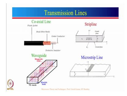
So, we start with transmission line. So, in that transmission line, we have a coaxial line. So, I am sure, most of you might have seen the coaxial. So, it has a center conductor, on that we have a dielectric insulator and then on that there is a metallic, you can say, sometimes a copper or even some times aluminium and followed by there is a plastic jacket on that. So, this whole unit becomes a coaxial line, then you might have also studied in the electro-magnetic course about waveguide.
