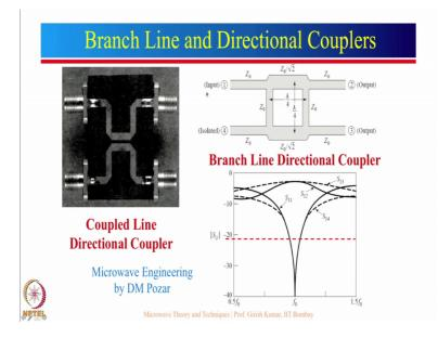
Then we will talk about the branch line and directional coupler. So, what you see that picture over here, you just imagine here, this is a 1 micro strip line which is going over here. So, we are feeding this input and this is the output. Now, what has been done here; another micro strip line has been put which is gap couple to this particular line now because of the fringing fields along this particular line part of the power gets coupled.
