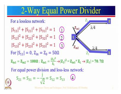
So, let us say if we are giving a input at this port here, then the half power should go here ideally and half power should go over here ideally and nothing should reflect back. So, where we need this kind of a power divider; for example just to mention one of the applications that if you want to feed let us say 2 element antenna. So, what will you do so we actually gave input at one place and then the power is divided equally and that is given to the 2 element.
