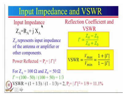
So, input impedance of any particular line or it can be of an antenna or an amplifier or other components can be defined in terms of real and imaginary terms R A and j X A. So, from this input impedance, we can find out the reflection coefficient. The reflection coefficient is given by Z A minus Z 0 divided by Z A plus Z 0.
