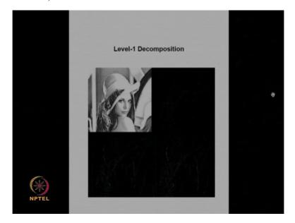
But it can be seen from the simulation here that as maximum energy or maximum information content is there in the LL subband so we would like to decompose this band further.
