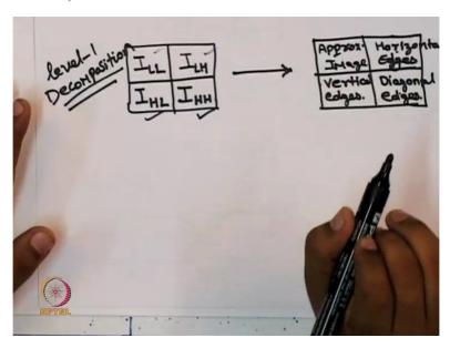
Therefore each of these subbands that is LL subband, LH subband, HL subband and HH subband contains only 1/4<sup>th</sup> of the total number of samples in our image originally. Now, in principle any one of these subbands or all of these subbands can be analysed or partitioned further.
