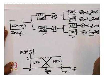
Since we have done subsampling by a factor of 2 both along the rows and along the columns, it means that in effect, we have done subsampling by a factor of 4.
