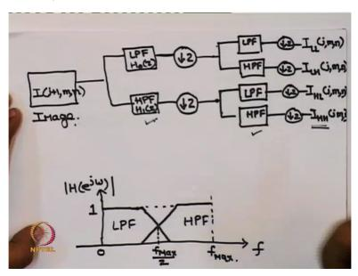
Now, it is important to observe here that the outputs subimages are at one resolution less than the image that we have started with. That is, we have in effect lost the resolution by a factor of 2 along the rows of the image and also along the columns of the image.
