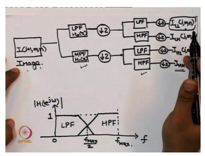
So if we perform the same operation as we have done for level 1 decomposition over here and take the output that we have obtained as ILL JMN and now consider this output as an input over here and perform the same operation that we have carried before we will get level 2 decomposition.
