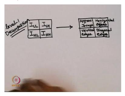
Pictorially, this can be represented as, this is our output that we have got as ILL. This is the subband where our output ILH will occur is our subband where the output IHL will occur, this is the subband that the output IHH will occur. This represents that in this part of the image or in this subband of the image we get an approximation version of the image.
