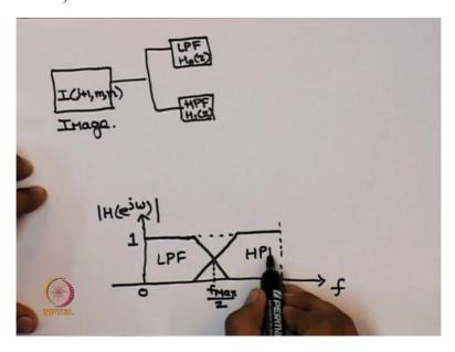
So let this be a much and let us the present this image by I with scale J+1 M and N, where M denotes the rows of the image and N denotes the column of the image. To start with, we can say that this image I is an original image itself and we will later see that this input I can be any signal and at any scale, J. So suppose, I J+1 MN is the starting signal and it is passed through two filters, one a low pass filter and a high pass filter with transfer functions of H0Z and H1Z respectively.
