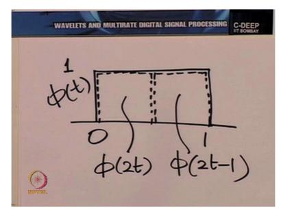
In fact, we can even say graphically. Indeed, you know if you recall, phi t looks like this. I've kind of scaled up the drawing. And all that you need to do to get this recursive equation is to notice that this can be redrawn like this. So, it has 2 components in it. And the  $1^{st}$  component is phi 2t and  $2^{nd}$ , phi 2t -1 and the whole thing is phi t. So we have a beautiful dilation equation which governs phi t.
