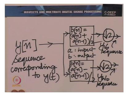
And if you pass it through 2 filters, the upper filter is described by the equation well you know, now I cannot use y n for the output because I am using y n to describe this. So I use different input output notations here. I will say in these 2 discrete time filters A is the input and B is the output. So I have B n is A n + A n - 1 by 2. And here I have B n is A n - A n - 1 by 2.
