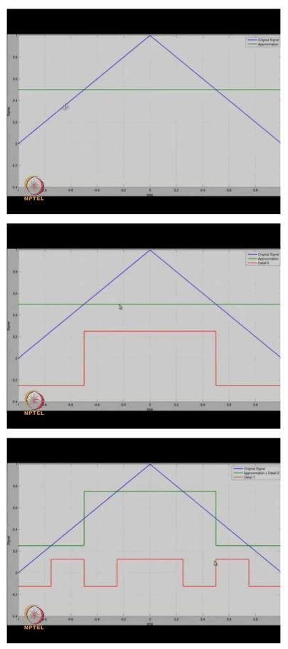
So let us have a look at another signal function which is a triangular function. The approximation to this function is shown in green and the original function is shown in blue. When we take the projection of the blue function on the W0 subspace, it looks like this and when we add this detailed function to the green approximation, what we obtain is a better approximation to the triangular function which looks something like this.
