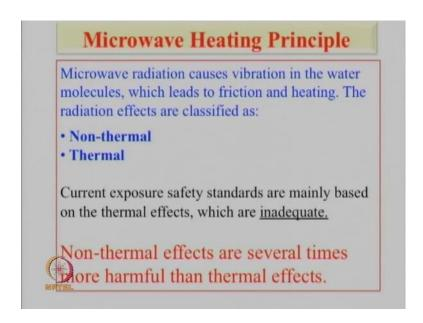
So, let us see what is the principle of microwave heating know when we put food inside a microwave oven that is the water in the fluid which is observing the radiation. So, what happens when microwave radiation impinges on the water molecule then the water molecule starts vibrating at a speed of 2.45 billion times per second and when that vibration is there at such an high intensity it leads to the friction and that friction leads to heating and that is how a microwave oven food gets cooked.
