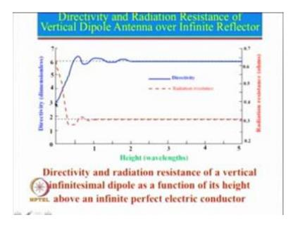
So, here is the plot of the directivity versus height as well as the radiation resistance. Let us first look at the directivity curve. So, one can see that when height is equal to 0 here then the directivity is equal to 3. The reason for that I just explained; that dipole is only going to radiate in the upper hemisphere. So, hence its directivity will increase by 2 times. So, for a normal small dipole antenna it is 1.5, for this case the directivity will become 3.
