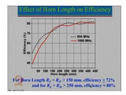
And then now let see the effect of the horn length. So, here aperture dimensions are fixed as before I mentioned I will just go back here. So, the aperture dimensions are 450 by 320. And what we are showing you is the effect of this particular horn length change.
