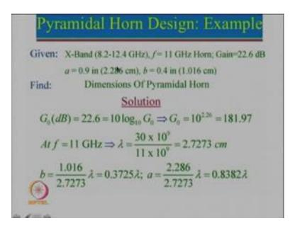
So, we actually just shown you this particular example. This example is again given in the Balanis book. So, here x band antenna is to be designed at poor that the first step is to choose the proper x band wave guide. Because that desired frequency at which antenna is to be designed this 11 gigahertz and the gain is 22 point 6 dB.
