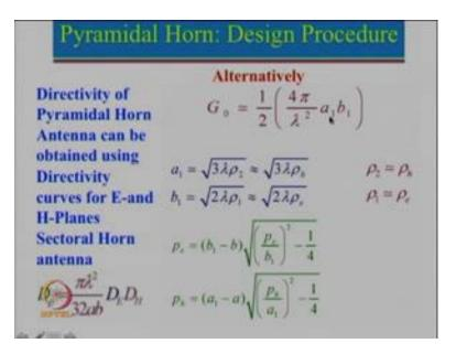
And then we had actually seen that the gain of the pyramidal horn antenna which has been taken as this particular term which is a 4 pi area divided by lambda square that is in normal directive expression, and area is here aperture area which is equal to a 1 times b 1.
