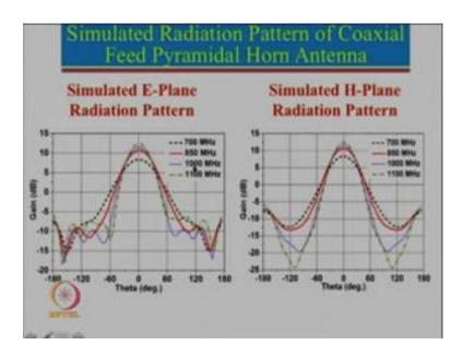
And let just also look at the radiation pattern. You can see the radiation pattern E-plane as well as H-plane, and here is the frequency value 700 850. We can see frequency is increasing, and this is the gain plot. You can see the gain is slightly increasing. So, that is a reason because aperture is fixed frequency is increasing and we know that the directivity is given by 4 pi a by lambda square. So, if the frequency is increasing lambda will reduce hence gain will increase.
