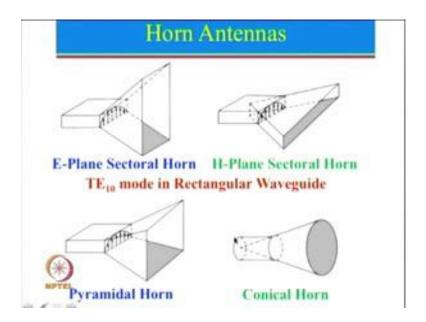
So, in the horn antennas these are the commonly used horn antenna. So, what are these here? There is actually a E-Plane Sectoral horn antenna, this is H-Plane Sectoral horn antenna and this is Pyramidal horn antenna.
