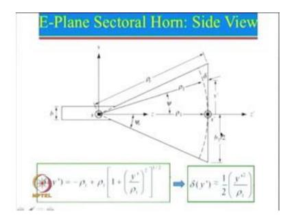
So, this is the side view of the Sectoral horn. So, from the side if we see we will see the dimension b, and then this is expanded in this particular plane here. The total dimension will be b 1 and this is b 1 by 2 and then you want to define the phase center of the horn antenna.
