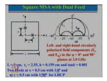
We had seen that here is a square patch and we had fed at 2 orthogonal points and by feeding this 1 angle 0 1 angle 90 degree which is this is 1 angle 0, this is 1 angle 90, we got LHCP, alternatively if you make 1 angle 0, 1 angle minus 90 then it will become RHCP.
