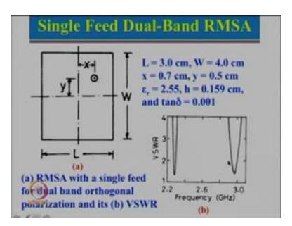
So, we had seen this configuration in the previous lecture by feeding along the diagonal. We could excite both the orthogonal mode. So, since width is large. So, this will be resonating at the lower frequency and since length is small this will resonate at higher frequency. And we saw this particular response here. So, instead of using a single feed point
