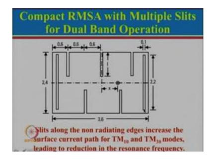
So, if you just see here this configuration is somewhat similar to the previous configuration. So, we have a rectangular patch and there are 2 slots over here, but now multiple notches have been cut. You can see here 3 notches have been cut over here and the 2 notches are cut over here, so there about 5 notches which have been cut along non radiating edges.
