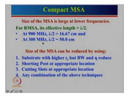
So, let us first look at the need. So, size of the micro strip antenna is large at lower frequency. For example, for RMSA, the effective length should be equal to lambda by 2. So, if you take an example of 900 mega hertz which fall under the category of GSM 900, when lambda by 2 is equal to 16.6 centimetre and if we have to design a antenna at let us say 300 mega hertz then lambda by 2 is 50 centimetre.
