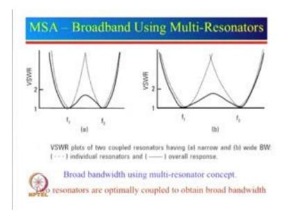
So, for example, let us say this is the VSWR curve for one of the antenna, which is resonating at f 1 if we now suppose excite another antenna which is resonating at frequency f 2, and if we do such a proper way of excitation and if we can now see that the overall curve will be a much broader curve, and if we look at a VSWR less than equal to 2 bandwidth, it will be much more than a single patch.
