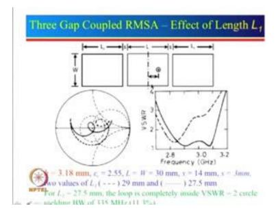
So, here the patches have been put along the non radiating edges, and one can now see that here we have a feed point and the patches are put on the other side over here.
