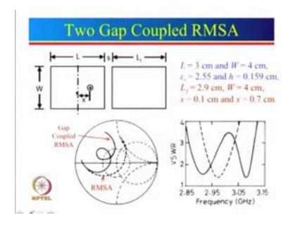
So, what we have here it is only one patch is fed, and these patch dimension we had taken earlier. So, we have kept same as the earlier dimension. So, which was L equal to 3 centimeter, W 4 substrate parameters are also same as before.
