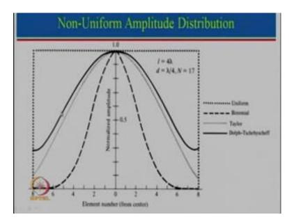
So, what are the different plots here let us just look into it. So, here is an non uniform amplitude distribution for different cases, but first one here is uniform; that means, all elements are fed uniformly. What we have taken here total number of elements 17. So, here are central element 8 elements on the right side, 8 elements on the left side. And the spacing here taken is lambda by 4. So, the total length of the array is 4 lambdas.
