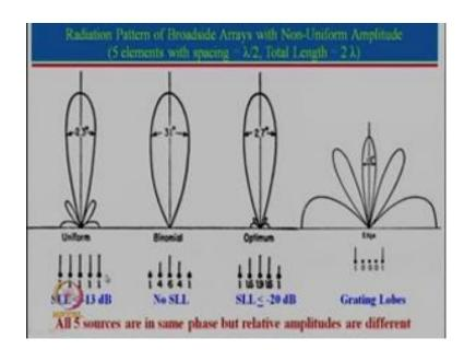
So, again let us take a case here there are 5 elements are there. So, for these 5 elements a equal amplitude is fed and the spacing between the element is lambda by 2. And if the spacing is lambda by 2 total lengths will be 2 lambdas from 1 to 5 elements. So, for this
