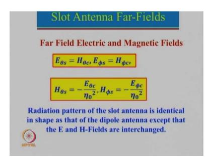
So, now for slot antenna far field electric and magnetic field will be exactly same as the dipole antenna with only one difference that, E field will be replaced by H field and H field will be replaced by E field. So, other than that everything remains same.
