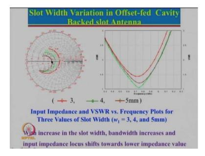
Now, here is the slot width variation. So, what we have done we have taken 3 different slots here 3, 4, 5 by changing the slot width the change in the resonance frequency is very small, but what we really see here is the change in the impedance plot is very very significant. So, for thin slot the bandwidth is actually less or we can say other way impedance is high. So, impedance variation will be more. So, which is given by this curve here and then the slot width is increased.
