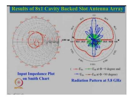
So, now let us what are the results. So, one actually got here for this particular array we got a decent matching you can see that it is centered around 50 ohm line over here we will see the measured and simulated VSWR here is the radiation pattern. So, we can see that in one plane there is a no change because we have not added array, but in the other plane you can see that this is the one main lobe and then there are lots of side lobe. One
