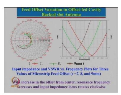
Here is the effect of the offset. So, if you change the offset now one actually wonders why if the offset is changed or the resonance frequency changes? The reason why resonance frequency is changing that this offset feed is placed on the slot. So, what is happening here now this is getting coupled along with this here. So, current distribution variation varies because of this loading.
