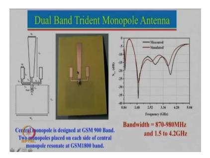
Now, let me show you one another configuration in parallel we worked on it this is actually dual band trident monopole antenna. So, what we have done here is we have designed a antenna at the center over here which resonates around again 900 mega hertz.
