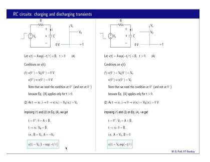
As our first example let us consider this simple RC series circuit. So, we have R and C in series and this combination is driven by a voltage source with a step voltage. So, this V s is 0 volts up to t equal to 0, and then it abruptly changes to V 0 and it remains constant after that point and we are interested in finding this capacitor voltage and the capacitor current as a function of time.
