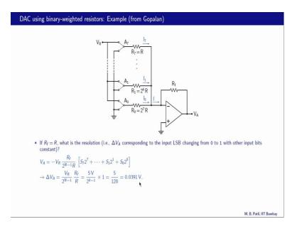
Next question, if R f is equal to R what is the resolution that is delta V A change in V A here corresponding to the input LSB changing from 0 to 1 with all other input bits kept constant all right. So, this is our expression for V A and this bracket corresponds to the input binary number, what is the lowest value of this bracket? That happens when S 0 is 0, S 1 is 0 etcetera all the way up to 7 equal to 0. So, that lowest value is 0 what is the
