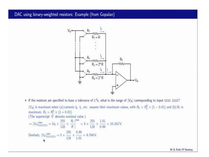
Next question, if the resistors are specified to have a tolerance of 1 percent what is the range of mod V A corresponding to the input 1 1 1 1 1 1 1 1 1. Now first let us figure out what this means a tolerance of 1 percent take this resistance for example, let us say it is
