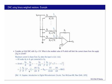
Let us take a specific example, consider an 8 bit DAC with V R equal to 5 volts, what is the smallest value of R? that resistance which will limit the current drawn from the supply to 10 milliamps, this is our supply V R and that is supplying all these currents and the total current that we draw from the supply it should be limited to 10 milliamps. Now since this is an 8 bit DAC our resistance values go from R, 2 R, 4 R etcetera then 2 raise to 6 R and the last value is 2 raise to 7 R.
