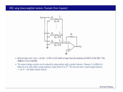
So, as we found in the last slide for a fixed input combination such as 1 1 1 1, 1 1 1 1 1 the output voltage can vary substantially because our resistances are not perfect they are nonzero tolerance and in the last example we found that the maximum V A in magnitude was 10.162 and the minimum was 9.764 and the difference between these 2 is about 0.4 volts which is quite significant because it is much larger than the resolution of the DAC which was 39 millivolts.
