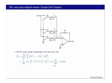
Next find the output voltage corresponding to the input binary number 1 0 1 0 1 1 0 1 fairly straight forward to do we have V A here, all we need to do now is to put S 7 equal to 1, S 6 equal to 0, S 5 equal to 1, S 4 equal to 0 and so on and that is what we get. So, V A turns out to be minus 6.758 volts.
