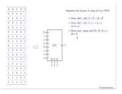
Let us consider this example. Implement the function X using an 8-to-1 multiplexer. Now in this case the function X is not given in the form of a logical expression, but it is given in the form of it is truth table here; so here is our 8-to-1 multiplexer that is the output X. These are the input lines I0 to I7 and these are the select lines. Now suppose we choose S2 equal to A S1 equal to B and S0 equal to C.
