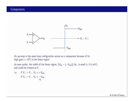
We will now look at some applications of Schmitt triggers, but before that let us talk about comparators, what is a comparator? It has 2 inputs plus and minus and 1 output, if V plus is higher than V minus then the output is high and if V minus is higher than V plus then the output is low and this figure here shows the relationship between V o and V plus minus V minus.
