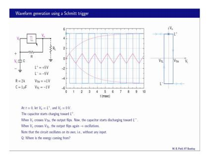
Let us take a look at this circuit, what do we have here? We have an inverting Schmitt trigger and that is its V o versus V i relationship and its reproduced here, this is the high tripping point V TH, low tripping point V TL - L plus is the high level of V o and L minus is the low level of V o, this axis is V o this axis is V i, V o is here and V i is here. So, V i is the same as the capacitor voltage.
