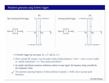
We will now look at another application of Schmitt triggers and that is to generate wave forms. In particular square wave output voltages here is a summary of the V o versus V i relationship for a non-inverting Schmitt trigger and an inverting Schmitt trigger and here are the symbols.
