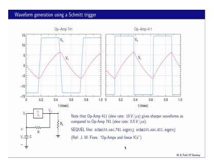
If you hookup this circuit in the lab you will realize that it cannot be pushed to arbitrarily high frequencies and that is because op-amps have a finite slew rate for example, op-amps 741 has a slew rate of 0.5 volts per micro second. This is the wave form obtained
