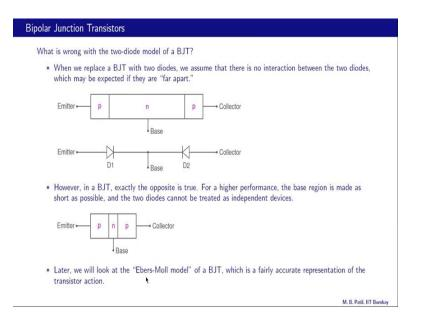
Let us now see what is wrong with the two-diode model of a BJT. Here is the two-diode model two-diodes connected back-to-back. What it implies is that this n region the base region is very long, and that these two junctions the emitter-base junction and the collector-base junction are far apart and that implies that there is no interaction between these two-diodes.
