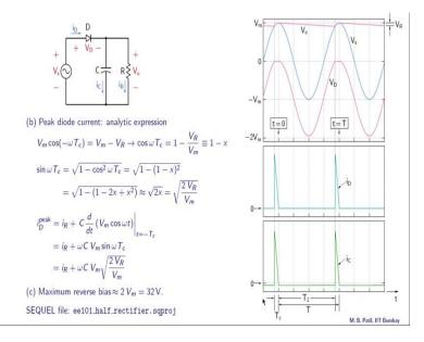
Let us now obtain an analytic expression for the peak diode current. We begin with this condition the source voltage at minus T c is equal to V m minus V R at that point we have seen that in the last slide and that gave us an expression for cos omega T c as 1 minus V R by V m. And earlier we calculated omega T c using a calculator got a numerical value for omega T c and then proceeded. Now, we want to do the same thing analytically.
