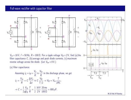
Here is a numerical example, and we have kept the numbers the same as the half-wave rectifier circuit. The maximum voltage input voltage is V m equal to 16 volts, frequency is 50 hertz again, the load resistance is 100 ohms and for the same ripple voltage of 2 volts, we want to find the filter capacitance, the average and peak diode currents and the
