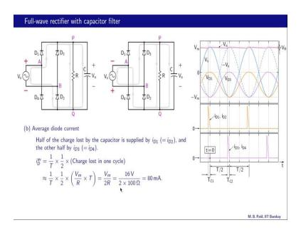
What about the average diode current. Now, as we observed earlier half of the charge lost by the capacitor is supplied by i D 1 or i D 2, because D 1 and D 2 conduct at the same time; and the other half is supplied by D 3 and D 4 that is this situation here. And therefore, we can write the average diode current let us say through D 1 is 1 over T times
