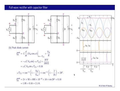
Let us look at the peak diode current and let us say we are talking about i D 1. So, i D 1 is maximum here. And as before this is the sum of i C and i R, because the current it is applying both the resistor and the capacitor. And the resistor current of course, we already know its approximately V m by R, and the capacitance current like in the half-wave case is the slope of this is given by the slope of this input voltage, and it is maximum at t equal to minus T c 1, so that is what we get.
