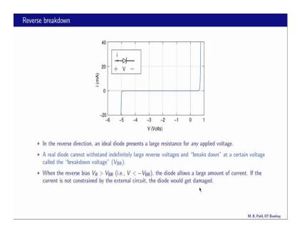
Let us now look at the i V curve of a real diode, and in particular we want to look at the reverse bias region; that means, with applied voltage less than 0 volts. In the reverse direction an ideal diode presents a large resistance for any applied voltage ideally infinite
