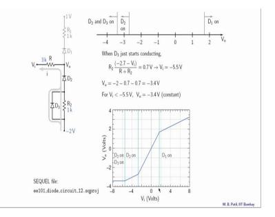
When D 3 starts conducting here two current paths: one through R 2 and one through D 3 like that. Now let us consider the case where D 3 has just begun to conduct; that means, this voltage is almost 0.7 volts, but not quite. So, this current is still 0 and this voltage drop is nearly equal to 0.7 volts. And in that case the current it is like that and we can use the expression that we derived for this current in the last slide; and that is given over here.
