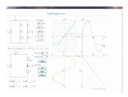
Next let us change this R 2 from 1 k to some very small value like 10 ohms leaving this V S 2 at minus 2 volts. In that case we do not expect the breakpoint to change because that is determined by the V S 2 and this voltage drop across the diode, but this slope will change because that is given by R 2 divided by R plus R 2.
