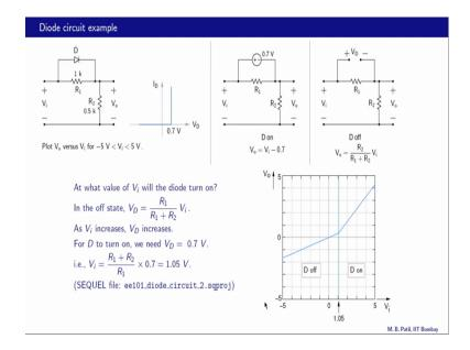
Here is our next diode circuit example, this is our input voltage V i that is the output voltage V o and we want to plot V o as a function of V i for V i varying from minus 5 volts to plus 5 volts. And this is the I D V D relationship for the diode that we will use, and it is of course the same as what we used previously.
