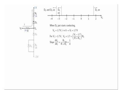
When D 1 conducts the current path is like that and in this situation D 2 and D 3 do not conduct, there is no current in this branch and therefore we have shown that in gray. Now as we have seen earlier D 1 starts conducting when V o becomes 1.7 volts. So, V o is 1.7 volts when D 1 just starts conducting and this current is still small so therefore this voltage drop is nearly 0. And in that case V i is equal to V o that is 1.7 volts, like that
