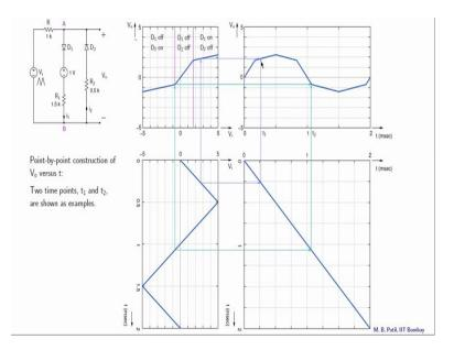
The next part of our problem is to find the V o as a function of time given a triangular input voltage varying from minus 5 volts to plus 5 volts with a frequency of 500 hertz. So, here is our input voltage wave form, this is the V i axis, this is the time axis: V i vary between minus 5 and 5 volts. And what we have shown here is 1 cycle since our frequency is 500 hertz the time period is 2 milliseconds and that is what we have over here 0 to 2 milliseconds.
