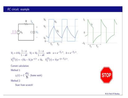
Here the results are summarized for the capacitor voltage; we have V 1 and V 2 here in terms of a and b, where a and b are given over here and once we know V 1 and V 2 we can find V c in the T 1 phase using this expression, and V c in the T 2 phase using this expression.
