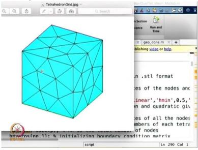
And we are getting the model and the model itself looks in this form it's a parallel plate capacitor but we are having a three-dimensional KCR so this is a top surface of the top conductor there is a bottom conductor and his other sides and as you can see they are going to be tetrahedral everywhere in our case before I explained it in a simplified manner in a paper where you see that is Q will have several number of tetrahedral.
