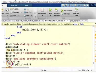
And we are calculating the element Coefficient matrix a as I explained before using this particular formula.
