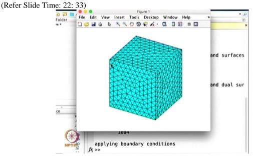
This is a very fine discretisation and as you can see we have gone from the initial problem of 0.5 as the minimum and maximum discretisation we have now 0.1 as the cell size the maximum size of the tetrahedral edges is going to be 0.1 and for this point discretisation we are able to get result which is also much more refined and this week and see in the result of the potential itself what you have computed.
