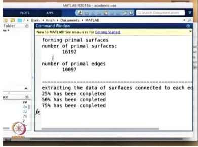
So you will see in the main window that we have 16192 surface 10097 Primal edges and we are extracting the data for the Primal surfaces edges and volumes and with that we will go and do the something for the dual edges dual volumes and dual surfaces and we are extracting the value and we are seeing the result.
