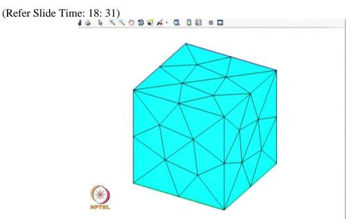
So this is the great that we are going to generate is surface has 1 2 3 4 5 6 7 8 9 10 11 12 13 14 roughly 14 or 15 tetrahedral and we are able to get to the point of seeing the result where we are able to simulate the problem for the potential .
