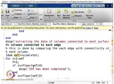
Now we are looking at the volumes and the connected edges. we are doing that to create the A1 A2 and A3 matrices if you remember the way we have to get the A1 A2 and A3 matrices depends on the connectivity and these are connectivity matrices and their connecting Each Other surfaces to the volume so we see volumes at each surfaces once we do that we are basically ready to generate the primal a1 matrix which is the matrix from edges 2 nodes.
