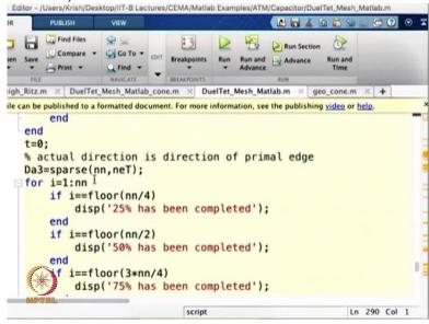
And we generate the dollar 3 matrix in a manner initially we declare it or initialise it as a sparse matrix this is very important step so as to make the code run faster
