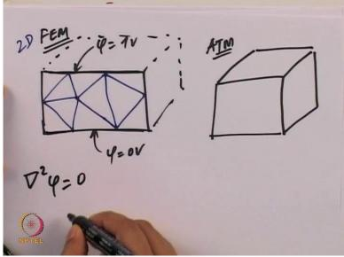
so let's start with the problem so we had this parallel plate capacitor which was in the case of the finite element method basically a 2D approximation and you said that of potential is 1 volte and the bottom potential is going to be zero volt so for us
