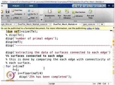
And we are also getting the information about Primal edges and we are going inside each of the surfaces to see the connected edges to the surfaces.
