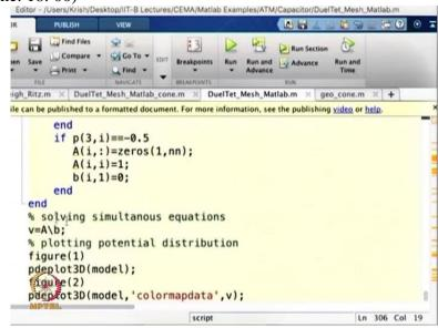
And you are solving the simultaneous equations initially we had we call to be where B is a boundary condition and we are able to solve for this equation by inverting the a and we are plotting the potential distribution for that problem so if you run this particular problem at the path what we will get is several information that we are interested.
