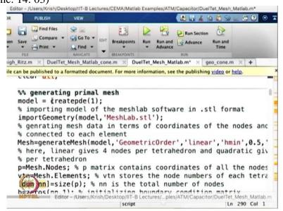
So we are generating the Primal grid using and in build program create PDE. (Refer Slide Time: 14: 15)
