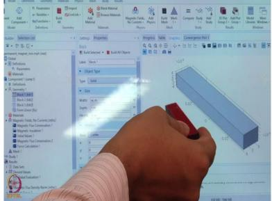
So this is the basic geometry you are using and the finite element solver you are using basically gives you the kind of geometry that you have modelled and you have taken basically the same dimension from the physical magnet you have and now you are going to mesh it, before that we will be enclosing it in a airbox.
