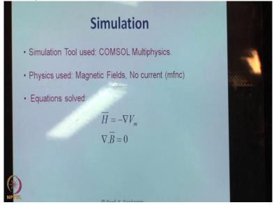
So basically you are starting to do the entire problem finite element solver. And you are modelling the thing with the scalar magnetic field. Ok! So H bar is basically the gradient of scalar magnetic equation J bar plus B bar and del dot B bar is 0. So these are the main equations which we will be plotting the magnetic fields.
