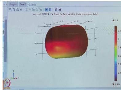
So what you are plotting here is the E field and then the reflector plane is pushing everything on the upside. Like (())(17:50) So the (())(17:56) is a bit shifted. ok So here the 0 is there there is a ground plane maximum is shifted here so what we can see is on the axis there is no (())(18:06).So this is classically like in (())(18:09). So this is the far field value of this particular antenna.
