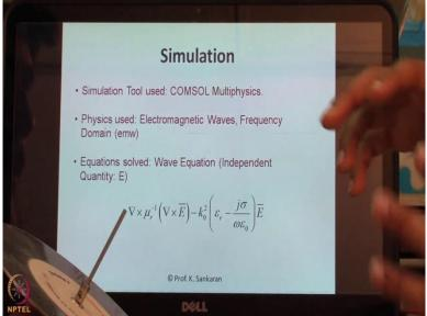
So in this type of simulation we saw a wave equation. ok and this equation we find the electirc fields all the points. Yeah So basically what you have is the wave equation as a curl formulation and its totally in terms of E. And what we have is the relative permeability and you have the sigma which is the conductance and then the omega and epsilon 0. ok. And came out is a wave number free space wave number. ok
