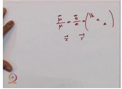
So let us go back anisotropy is in the Epsilon by Epsilon is equal to Mu by Mu we said if it is a x oriented PML we will have the anisotropy in this direction. And the rest it's a diagonal matrix and we will have 1 by an if it's an x oriented PML. So what we are trying to do is we are trying to make sure that this 1 will be the anisotropic direction will be instead of x it will be the radial direction. So instead of x we are going into the radial direction. (Refer Slide Time: 09: 31)
