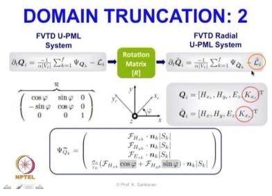
as you can see here in the earlier slide when Phi is 0 this component the Y component will become zero but this component will be there which is exactly the same as in the case of uniaxial oriented PML.
