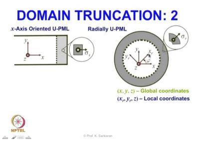
So right now we have got a simple condition where PML is sitting on the X axis. So the PML is actually an X oriented PML. So X axis oriented uniaxial PML. So what we want is we wanted to have a PML that is radially oriented. So in that sense regardless of which direction I am coming from the anisotropy which we called.
