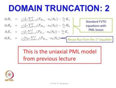
If you remember we had this equation that is coming from our system of equation of Finite volume, let us see this in this slide. We said that we can reuse the first flux directly computed from the first equation
