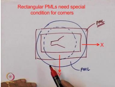
So in this kind of case what we want is we want to truncate the antenna like this. So in the case of a rectangular truncation we have to put the boundary conditions like this. But in case of a radial truncation our PML will be in this area. So this will be the PML area in the case of radial truncation in the case of rectangular domain this will be the PML. And also we already
