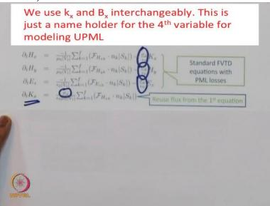
So irrespective of the fact that we have 4 equations, the last equation's the flux value is recomputed. And the first three is nothing but the standard Finite volume time domain equation with PML losses. And the losses are given using the terms here. And these terms are going to be the losses in the x direction. Because we were interested in truncating the domain main wave application or wave guide application along x axis. You can also notice that this
