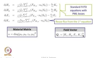
We said we will have the matrix material parameter given by alpha which is here as you can see in the slides. And these values are Mu 0 and Epsilon 0 accordingly and the field vector the combine field is given by Q i which is H x H y E z and K x. We are talking about transverse magnetic case the counterpart will transverse electric case where you will have E x E y and H z and accordingly the fourth value will also change.
