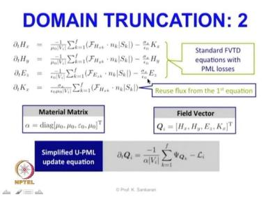
So we have the final form of the simplified equation which is given by the final equation here. As you can see this is semi discrete this is continuous still in time. But we have already covered how to discretise the time variable. So it is enough that we focus now on this one. So this L i are these loss terms. Let me explain further in the slide here.
