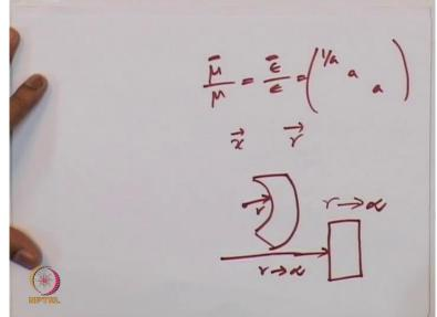
So if you can see here so this is the way we define the radius of curvature. So if we have a PML like this so this is the radius of curvature. So when r is tending to infinity so this will become almost flat. So here r is going to infinity so this is the kind of transformation or approximation we are tend into.
