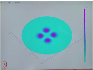
And we simulated various mode profiles for this multi mode fibre.
