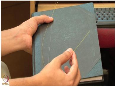
So these are as we said before they are designed for certain frequency, mainly designed for 1300 nanometre So you can go up with 300 mainly there are three optical windows are there one is 50 nano meter is there other one is 1300 nanometre is there and the third one is 350 nanometer. This 1300 nanometer is (())(05:05) So we are mainly using this for last long distance communication we are using 1300 or any window can be used.
