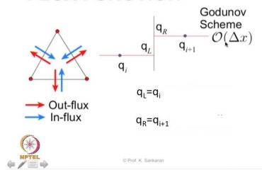
So the consequence of this is basically what I have shown here in the slide. So what is happening is we can say that it is a piece wise constant. We will see in the 2D how it will be in the next slide. But this is a kind of a constant approximation. Whatever is on the left so here qL is equal to q i and q R is equal to q i plus 1, where i and i plus 1 are nothing but bary centric values on the left and right hand side. And as I marked here this is of first order approximation.
