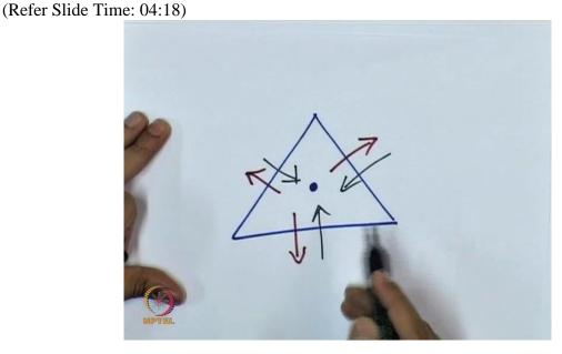
So when you consider a particular problem for example you have a triangle and this is your control volume and the values are in the centre and this control volume will have fluxes that are going in and out. So whatever is going out I mark it in red. And there is also fluxes that are going inside. So we said that the net flux will be the algebraic sum of those ingoing and outgoing flux.
