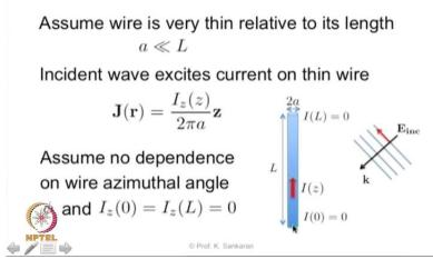
And now assume that there is no dependence on the wires azimuthal angles which is given by the Phi and Iz of 0 where when we start with the point here and at this point the current goes to 0, so the current goes to 0 at this terminal and at the other terminal.
