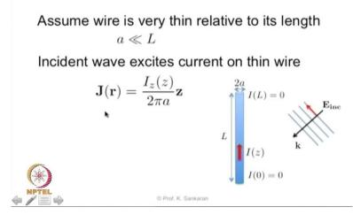
What we have is an incident wave that is coming with direction of propagation given by the vector k and the incident electirc field as certain orientation and it is going to be incident on this particular wire. What we see is the incident wave excites the current on this thin wire. So what happens here is the J(r) is going to be given by the expression Iz which is function of the z axis divided by 2Pir where r is equal to the radius a and z of course is the direction of the J vector.
