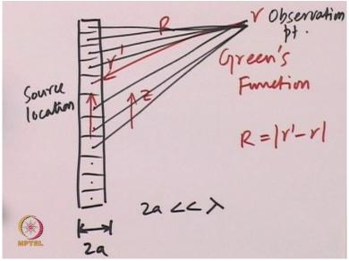
As I said the Green function is a response function to a source that is located at a particular location r prime and we are looking at the response of that source at r which is the observation point. In the case of the thin wire antenna we are going to sum up all the Green's function response and then going to the overall response. So let us start with the wave equation which is the for a z axis oriented thin wire antenna.
