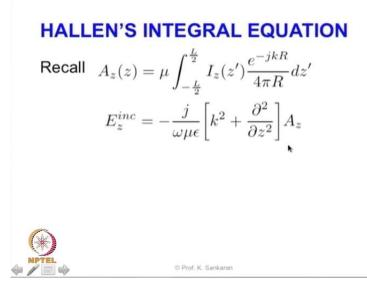
Remember that we used A z as a line integral which goes from minus l by 2 to plus l by2 and the value I z is the current that is flowing in that particular point z prime. And we are going to multiply it using the Green's function here. And then we are integrating it along d z. And once we have that we can substitute the value in the E incident expression for the Az.
