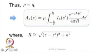
So with that what we have done here is transformed the entire equation from a volume integral to a surface integral to essentially a line integral.
