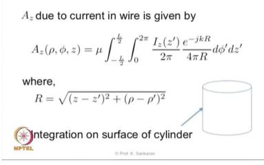
And now when we substitute the value for r which is located at a distance r from the point of the source itself. remember the source locations are given by z prime and rho prime. And the value of r is equal to the square root of z minus z prime square plus Rho minus Rho prime square so the integration is done on the surface of the cylinder as I mentioned.
