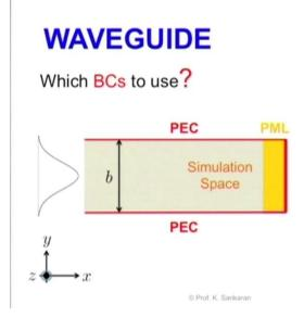
And waveguides simulations.
