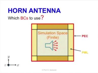
We demonstrated that epicacy and accuracy of the PML technique for a couple of practical applications namely horn antenna.
