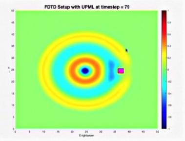
As an example we demonstrated using scattering applications with a point source incident on a scatterer.
