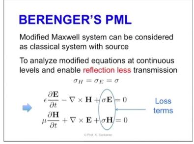
We examined the role of Loss E terms in the update equation and how one can optimise these losses for equipped PML performance.
